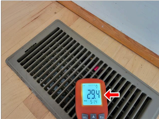
2.10.B Item 1(Picture) 29.4 Degrees (Supply Air)
