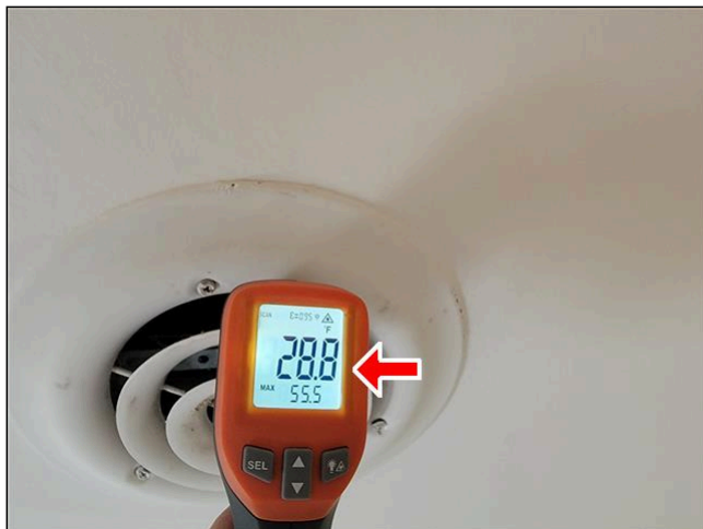
2.10.A Item 1(Picture) 28.8 Degrees (Supply Air)
