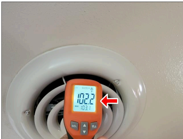
2.1.A Item 1(Picture) 102.2 Degrees (Heat Stage 1)
