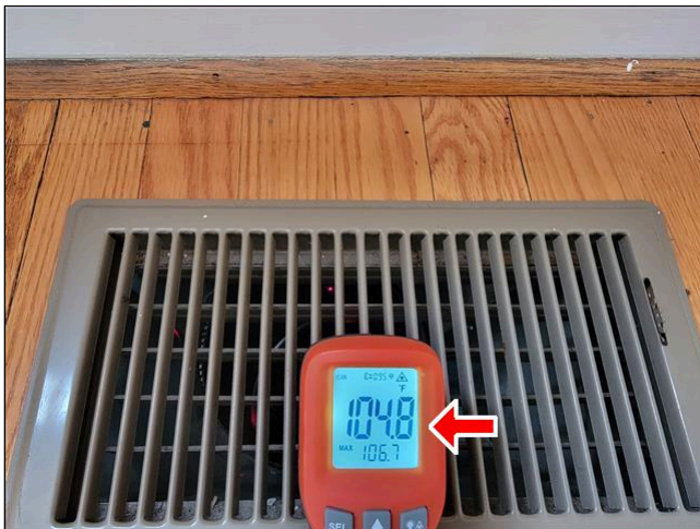
2.1.B Item 1(Picture) 104.8 Degrees (Heat Stage 1)
