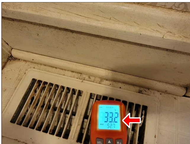
2.10 Item 1(Picture) 33.2 Degrees (Supply Temperature)
