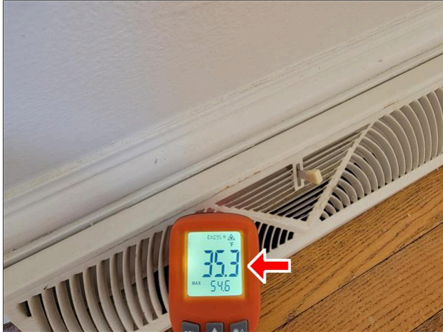
2.10.B Item 1(Picture) 35.3 Degrees (Supply Temperature)
