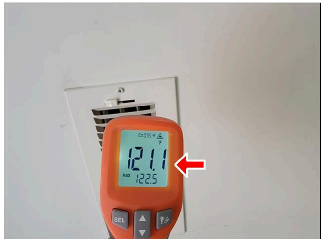
2.1.A Item 2(Picture) 121.1 Degrees (Heat Stage 2 "Aux")
