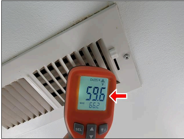
2.10.A Item 1(Picture) 59.6 Degrees (Supply Temperature)
