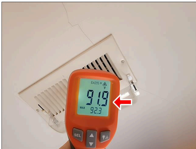
2.1.A Item 1(Picture) 91.9 Degrees (Heat Stage 1)
