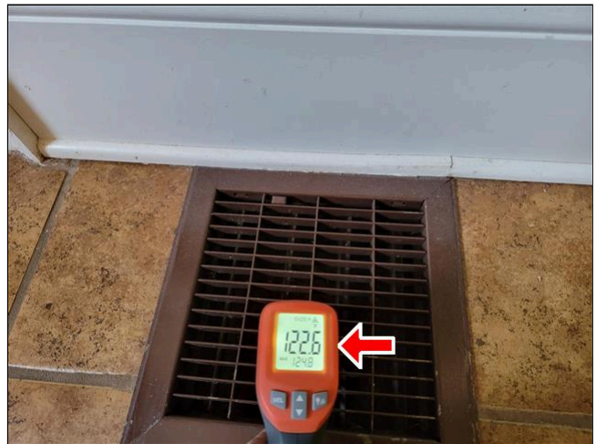
2.1.B Item 2(Picture) 122.6 Degrees (Heat Stage 2 "Aux")
