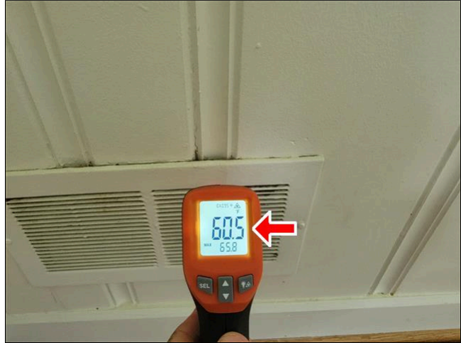
2.10 Item 2(Picture) 60.5 Degrees (Return Temperature)
